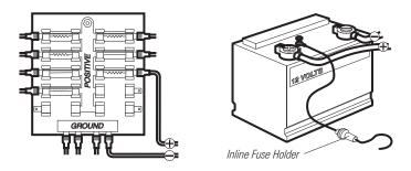
**CAUTION:** Some boats have 24 or 36 Volt electrical systems. Make sure that your HDR 650 is connected to a 12 VDC power supply. Use a voltage conditioner for variable inputs.
