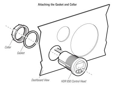
Hand-tighten the collar until the HDR is securely mounted in the dashboard. Make sure that the face of the HDR stays oriented upright. Hand-tightening the Collar
